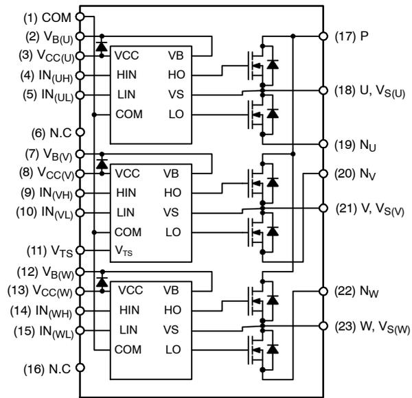
4. Source Terminal of Each Low-Side MOSFET is Not Connected to Supply Ground or Bias Voltage Ground Inside Motion SPM 5 product. External Connections Should be Made as Indicated in Figure 3.
