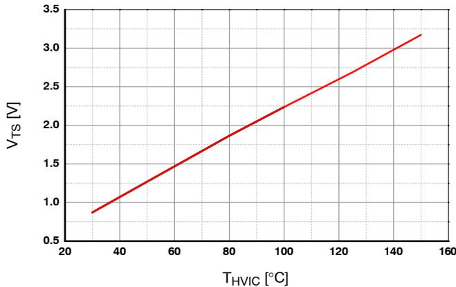
**Figure 5. Temperature Profile of V<sub>TS</sub> (Typical)**
