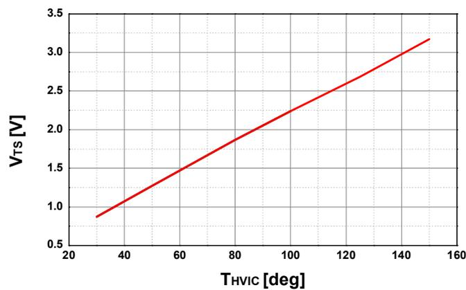
**Figure 5. Temperature profile of V<sub>ts</sub> (typ.)**
