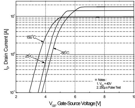
Figure 2. Transfer Characteristics
