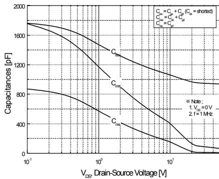
Figure 5. Capacitance Characteristics
