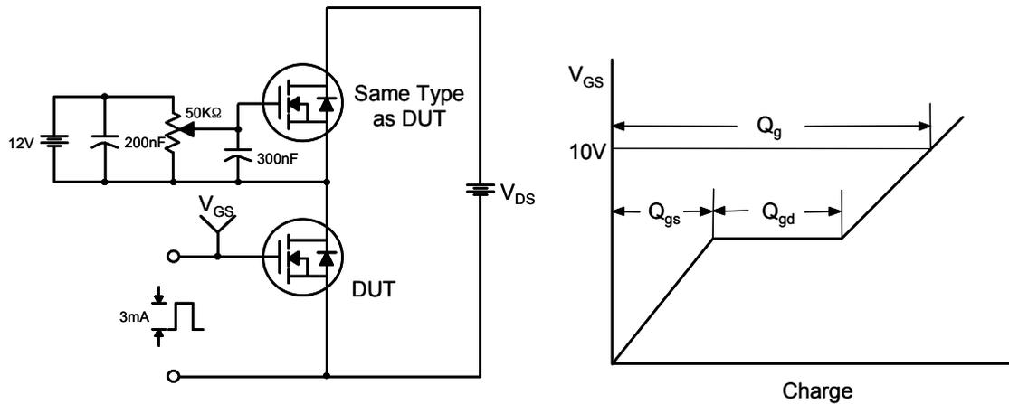
Figure 13. Resistive Switching Test Circuit & Waveforms
