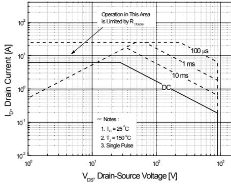
**Figure 9-1. Maximum Safe Operating Area for FQP8N90C**
