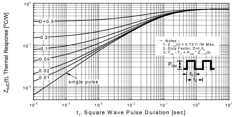
Figure 11-1. Transient Thermal Response Curve for FQP8N90C
