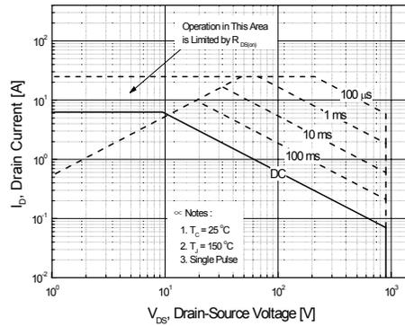
**Figure 9-2. Maximum Safe Operating Area for FQPF8N90C**
