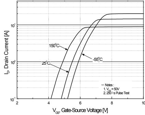
Figure 2. Transfer Characteristics
