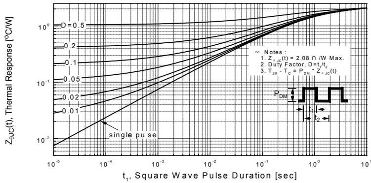
Figure 11-2. Transient Thermal Response Curve for FQPF8N90C
