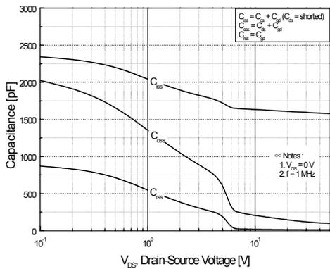
Figure 5. Capacitance Characteristics
