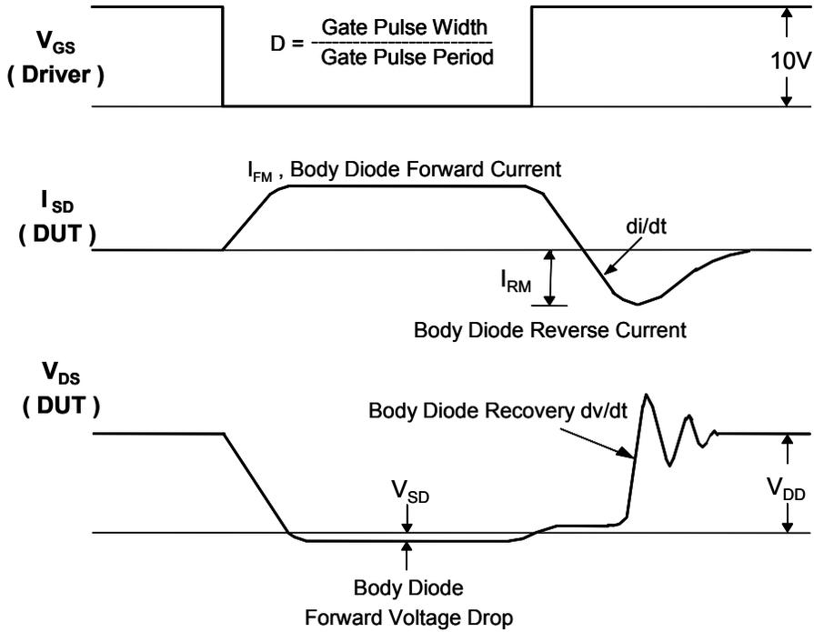
Figure 15. Peak Diode Recovery dv/dt Test Circuit & Waveforms
