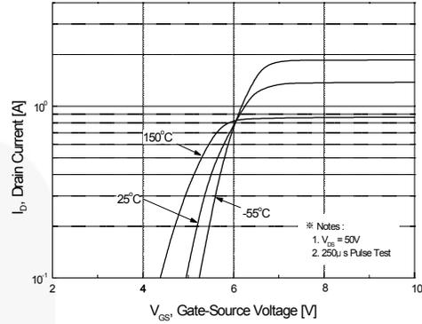
**Figure 2. Transfer Characteristics**
