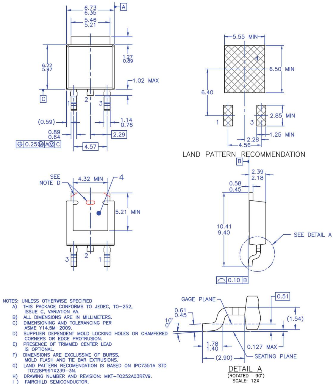
**Figure 16. TO252 (D-PAK), Molded, 3-Lead, Option AA&AB**
