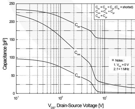
**Figure 5. Capacitance Characteristics**
