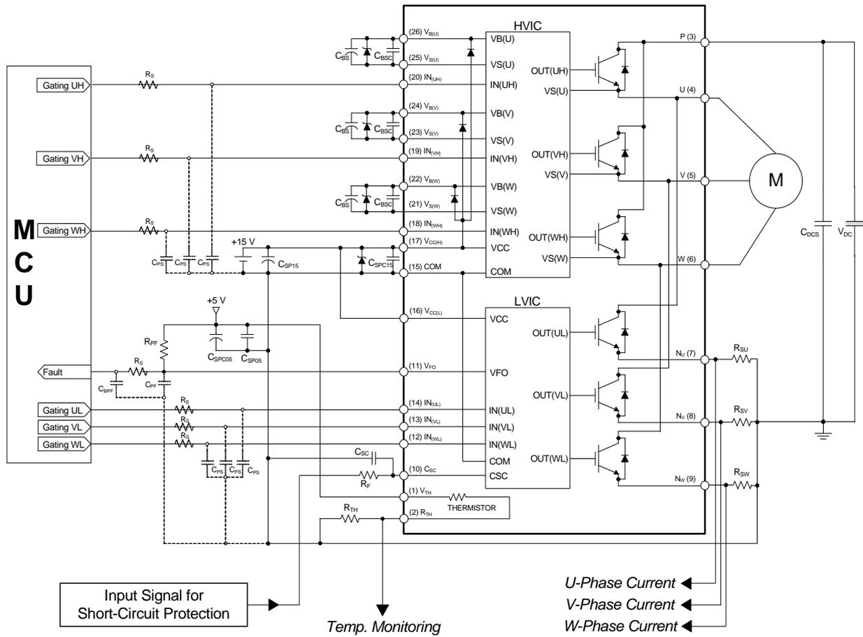
**Figure 15. Typical Application Circuit**
