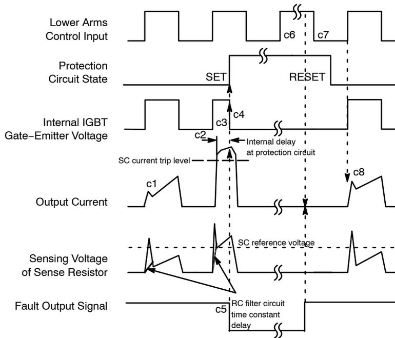
(with the external sense resistance and RC filter connection)
