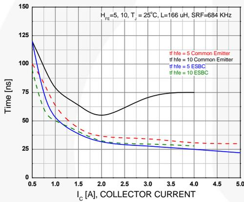
Figure 12. Inductive Load Collector Current Fall - Time ( $t_f$ )
