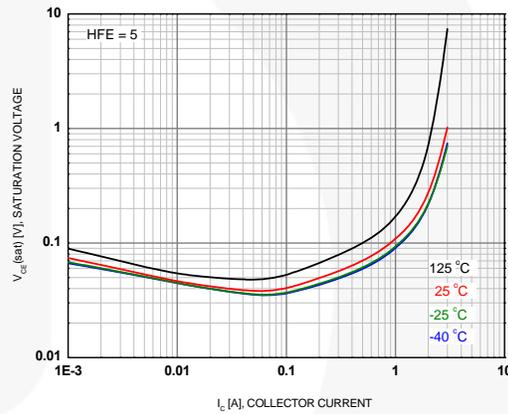
Figure 7. Collector-Emitter Saturation Voltage
