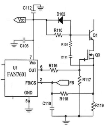
Figure 31. V<sub>CC</sub> Derived
