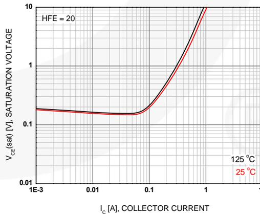
Figure 9. Collector-Emitter Saturation Voltage
