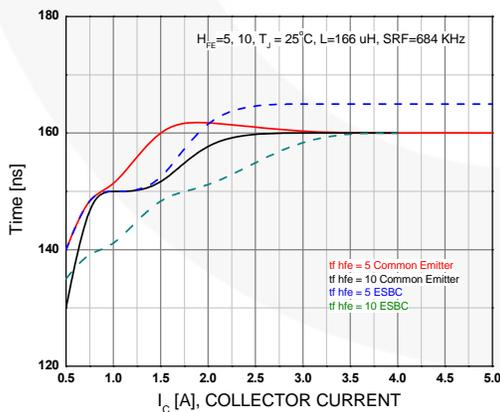
Figure 14. Inductive Load Collector Voltage Fall - Time ( $t_f$ )
