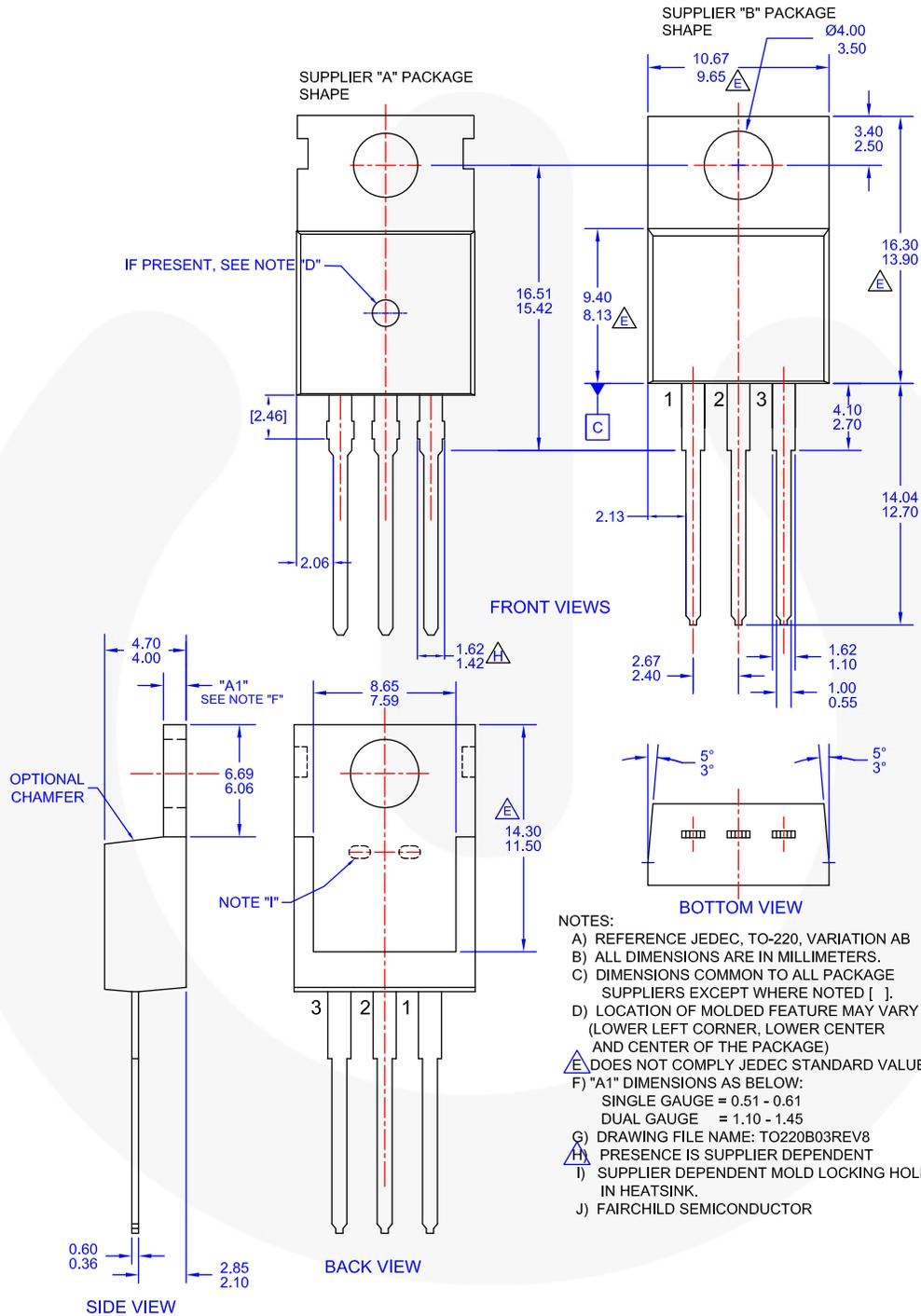
Figure 34. TO-220, MOLDED, 3-LEAD, JEDEC VARIATION AB
