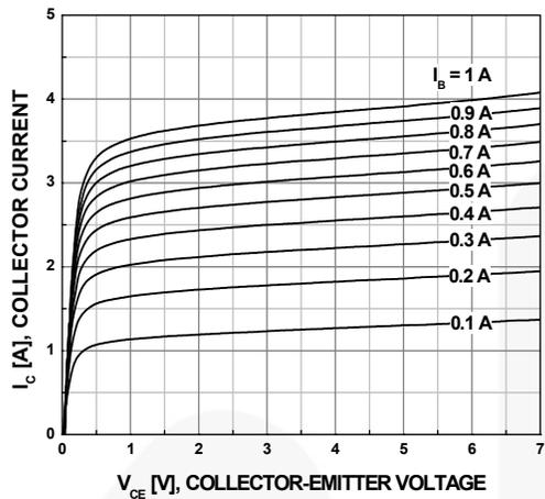
Figure 4. Static Characteristics
