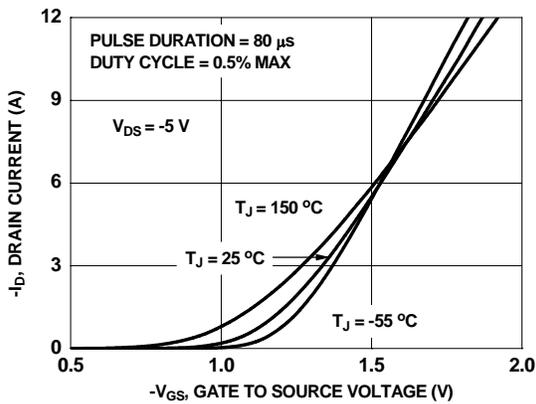
**Figure 5. Transfer Characteristics**
