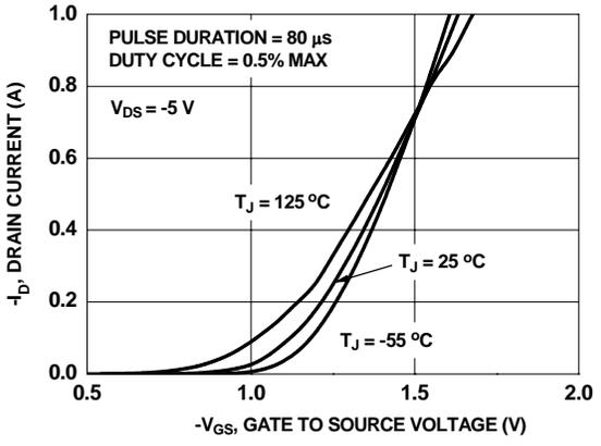
**Figure 5. Transfer Characteristics**
