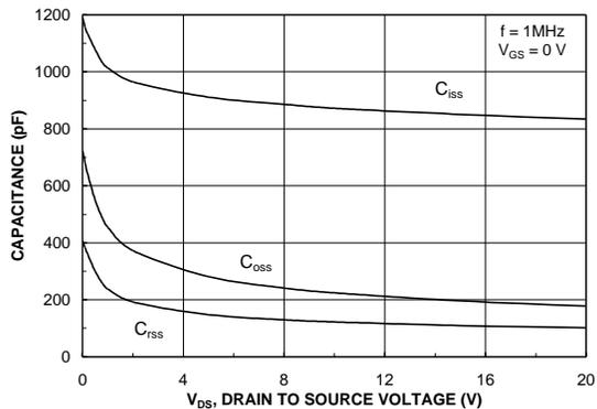
Figure 8. Capacitance Characteristics.
