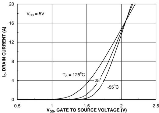
Figure 5. Transfer Characteristics.
