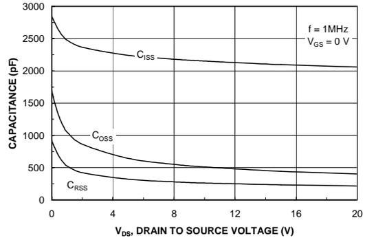
Figure 8. Capacitance Characteristics.
