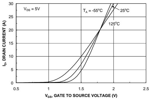
Figure 5. Transfer Characteristics.
