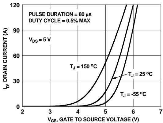
**Figure 5. Transfer Characteristics**
