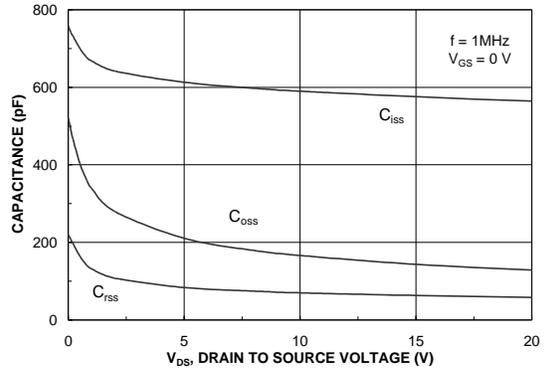
Figure 8. Capacitance Characteristics.
