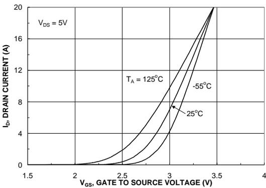
Figure 5. Transfer Characteristics.
