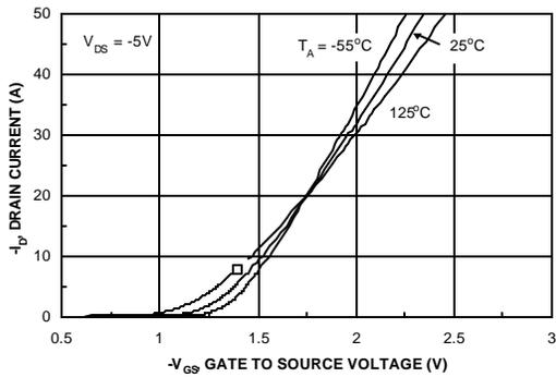
Figure 5. Transfer Characteristics.
