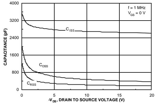
Figure 8. Capacitance Characteristics.
