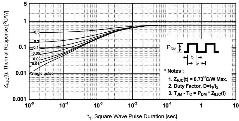
Figure 13. Transient Thermal Response Curve - FDPF12N50NZ
