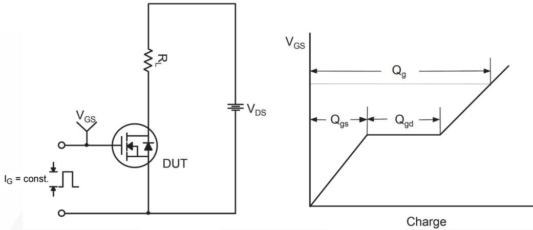
**Figure 15. Resistive Switching Test Circuit & Waveforms**
