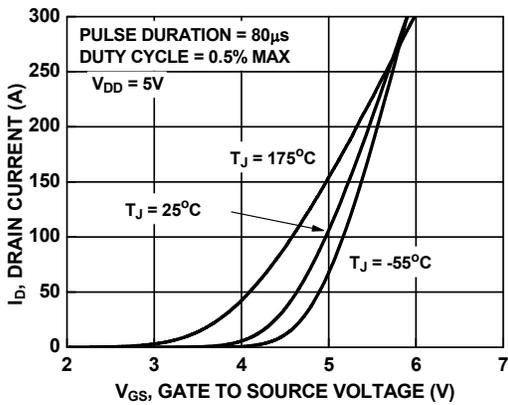
Figure 7. Transfer Characteristics
