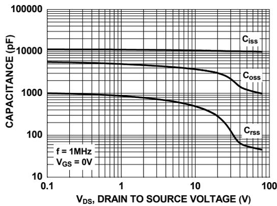
Figure 15. Capacitance vs. Drain to Source Voltage
