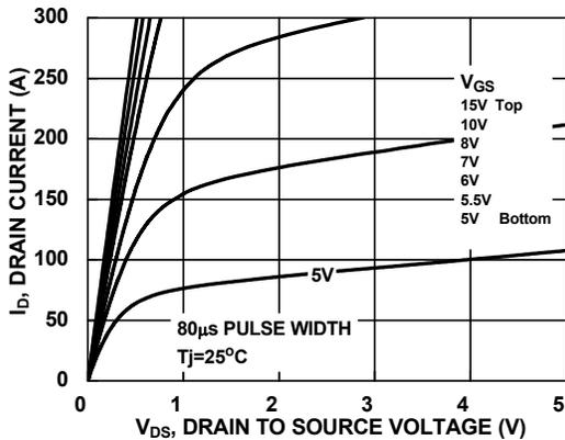
Figure 9. Saturation Characteristics
