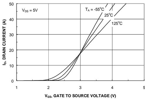
Figure 5. Transfer Characteristics.
