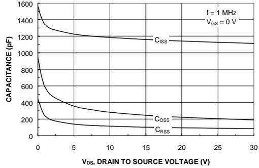
Figure 8. Capacitance Characteristics.
