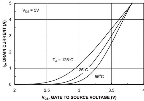
Figure 5. Transfer Characteristics.
