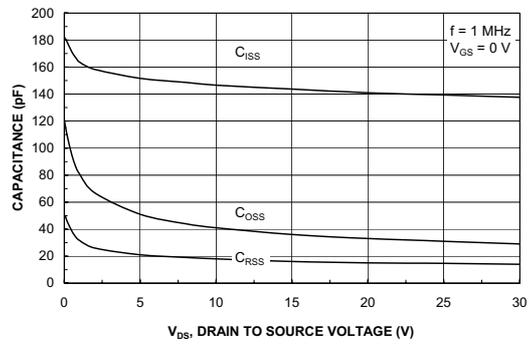
Figure 8. Capacitance Characteristics.
