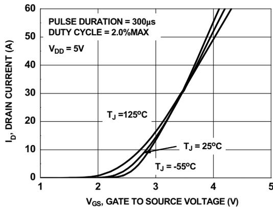
Figure 16. Transfer Characteristics
