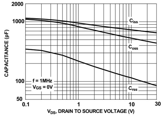
Figure 19. Capacitance vs Drain to Source Voltage
