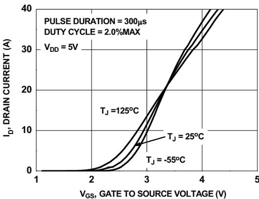
**Figure 5. Transfer Characteristics**
