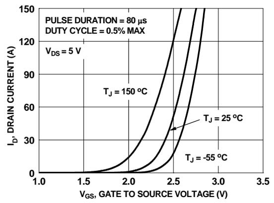
Figure 5. Transfer Characteristics
