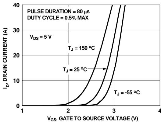
Figure 5. Transfer Characteristics
