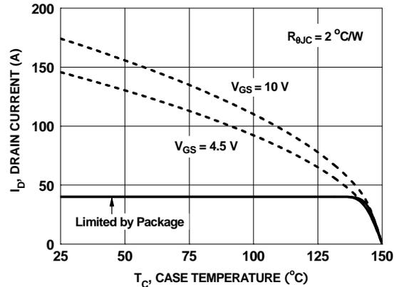
**Figure 23. Maximum Continuous Drain Current vs Case Temperature**
