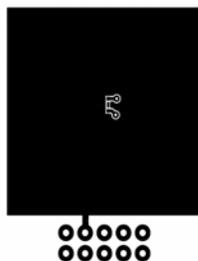
a.  $60\text{ }^\circ\text{C}/\text{W}$  when mounted on a  $1\text{ in}^2$  pad of 2 oz copper.
