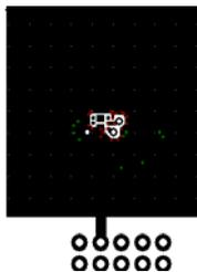
a. 90  $^\circ\text{C}/\text{W}$  when mounted on a 1 in<sup>2</sup> pad of 2 oz copper.
