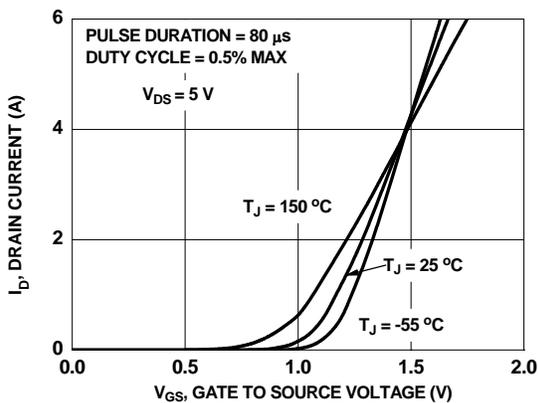
**Figure 5. Transfer Characteristics**
