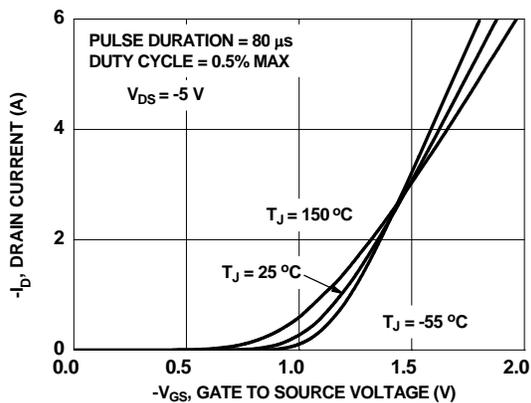
Figure 5. Transfer Characteristics
