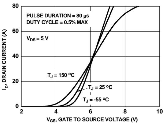
Figure 5. Transfer Characteristics
