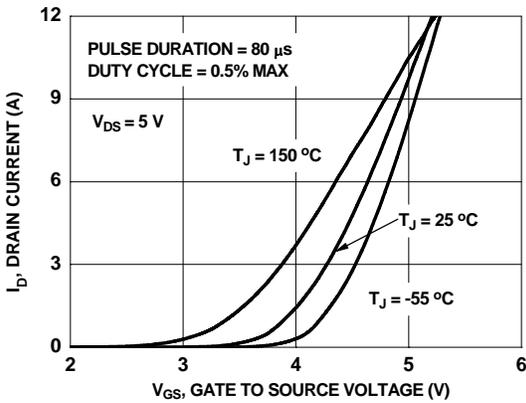
Figure 5. Transfer Characteristics
