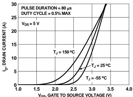
Figure 5. Transfer Characteristics
