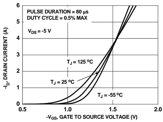
Figure 5. Transfer Characteristics
