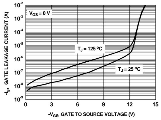
**Figure 9. Gate Leakage vs Gate to Source Voltage**
