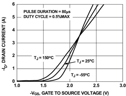
Figure 5. Transfer Characteristics
