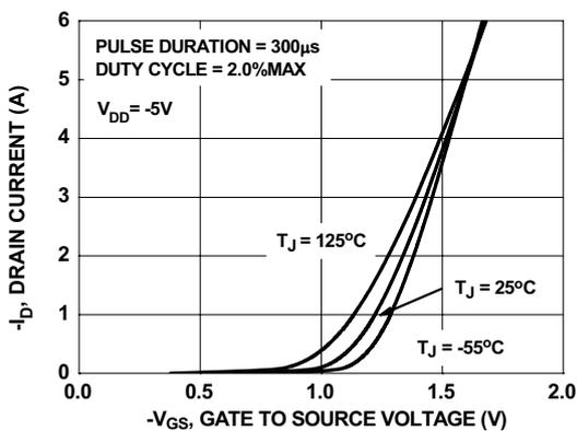
Figure 5. Transfer Characteristics
