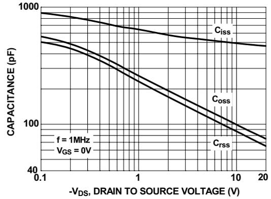
**Figure 8. Capacitance Characteristics**
