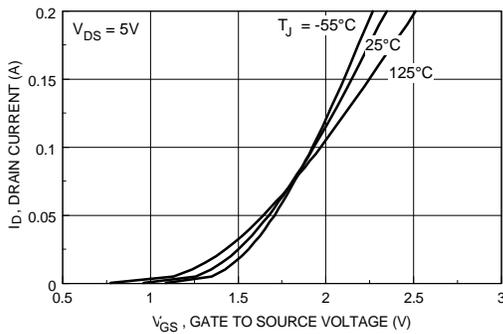
Figure 5. Transfer Characteristics.
