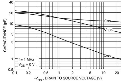
Figure 18. Capacitance Characteristics.
