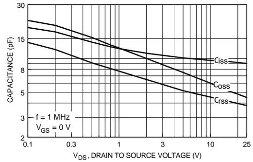
Figure 8. Capacitance Characteristics.
