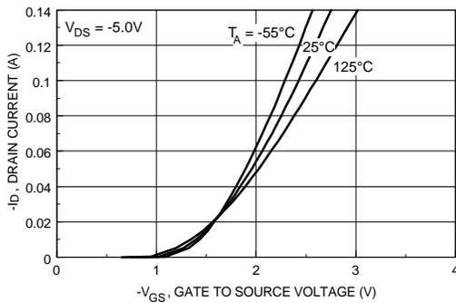
Figure 15. Transfer Characteristics.
