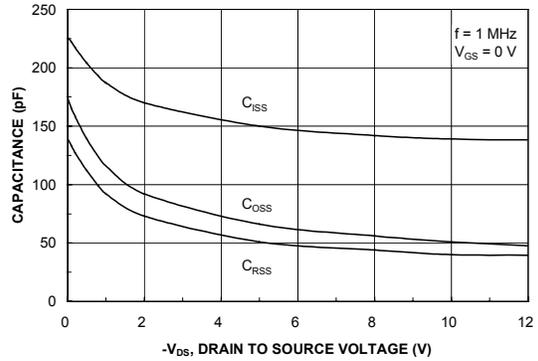
Figure 8. Capacitance Characteristics.
