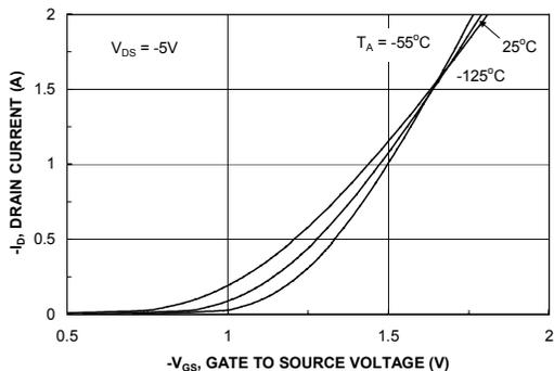
Figure 5. Transfer Characteristics.
