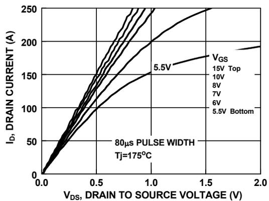
Figure 10. Saturation Characteristics
