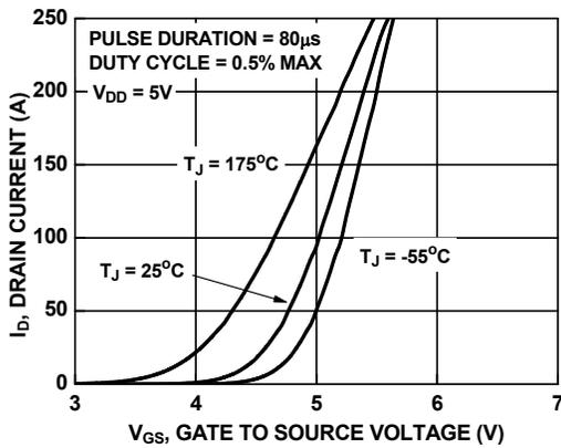
Figure 7. Transfer Characteristics
