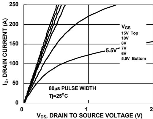
Figure 9. Saturation Characteristics
