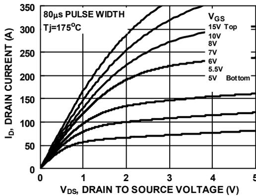
Figure 10. Saturation Characteristics
