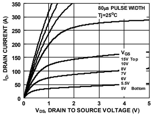
Figure 9. Saturation Characteristics
