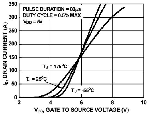
Figure 7. Transfer Characteristics
