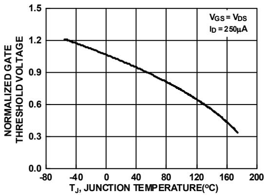
Figure 13. Normalized Gate Threshold Voltage vs. Temperature
