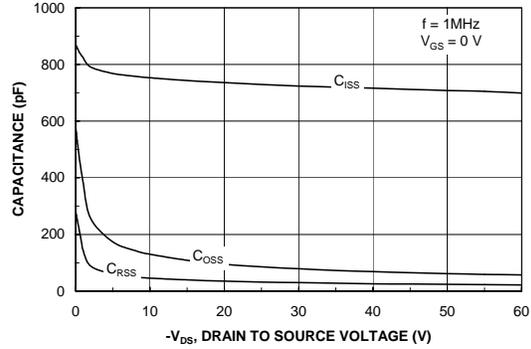
Figure 8. Capacitance Characteristics.
