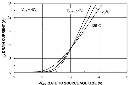
Figure 5. Transfer Characteristics.
