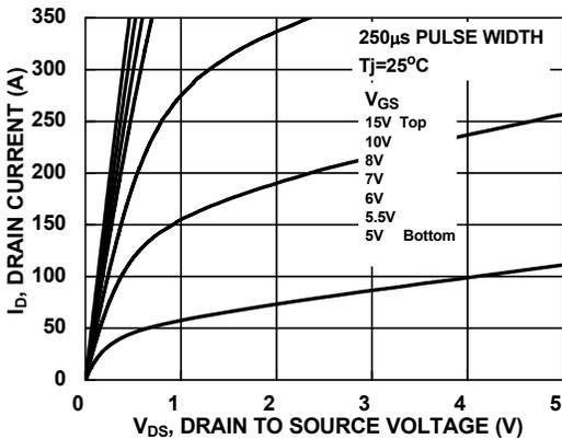
Figure 9. Saturation Characteristics
