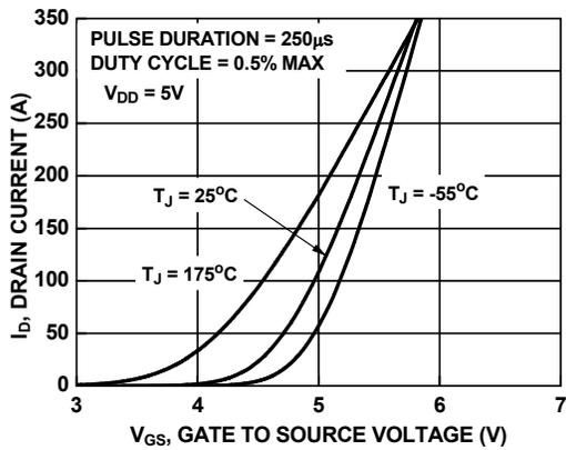
Figure 7. Transfer Characteristics
