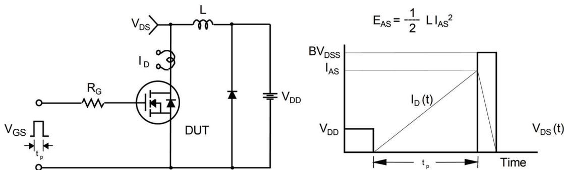
**Figure 17. Unclamped Inductive Switching Test Circuit & Waveforms**
