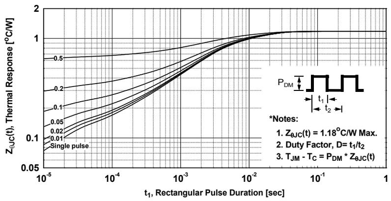
Figure 14. Transient Thermal Response Curve FOR FCPF380N60E
