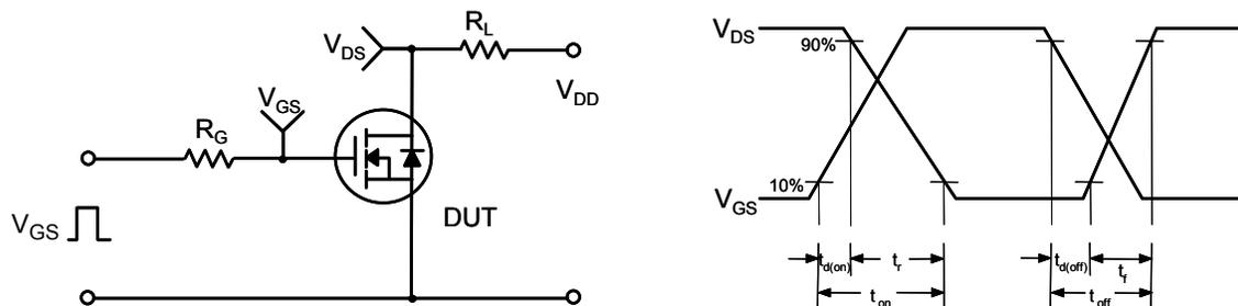
**Figure 16. Resistive Switching Test Circuit & Waveforms**
