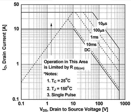
**Figure 10. Maximum Safe Operating Area for FCPF380N60E**
