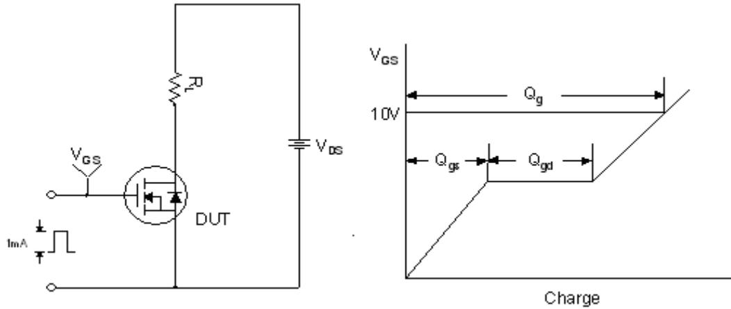
Figure 13. Gate Charge Test Circuit & Waveform
