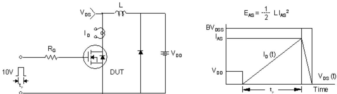
Figure 15. Unclamped Inductive Switching Test Circuit & Waveforms
