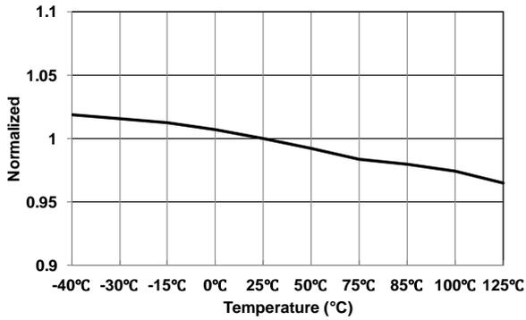
**Figure 3 Turn-On Threshold Voltage (V<sub>DD-ON</sub>) vs. Temperature**
