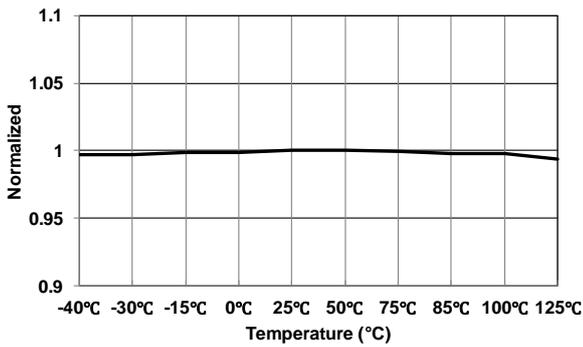
**Figure 5 V<sub>DD</sub> Over Voltage-Protection Level (V<sub>VDD-OVP</sub>) vs. Temperature**
