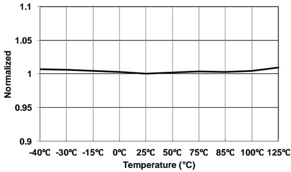
**Figure 17 Ratio between Threshold Voltage and Source Current ( $Z_{SD-TH}$ ) vs. Temperature**
