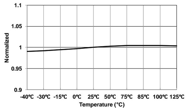
**Figure 8 Minimum Blanking Frequency (f<sub>BNK-MIN</sub>) vs. Temperature**
