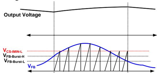
Figure 21 Burst-Mode Operation
