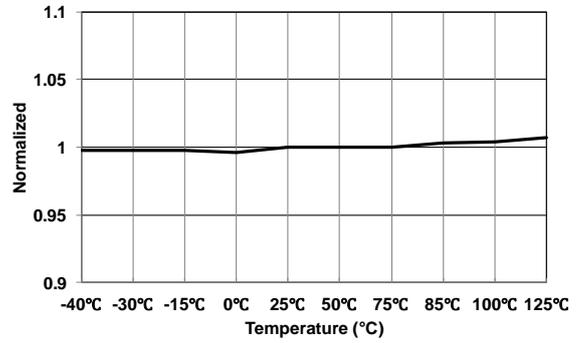
**Figure 4 Turn-Off Threshold Voltage (V<sub>DD-OFF</sub>) vs. Temperature**
