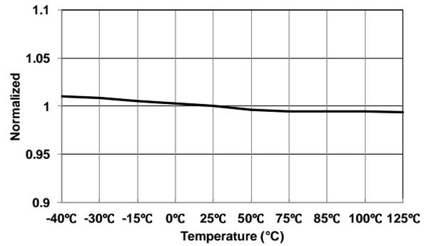
**Figure 20 Maximum On Time ( $t_{ON-MAX}$ ) vs. Temperature**
