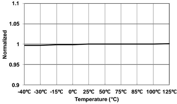
**Figure 15 Current Limit Threshold Voltage ( $V_{CS-LIM}$ ) vs. Temperature**
