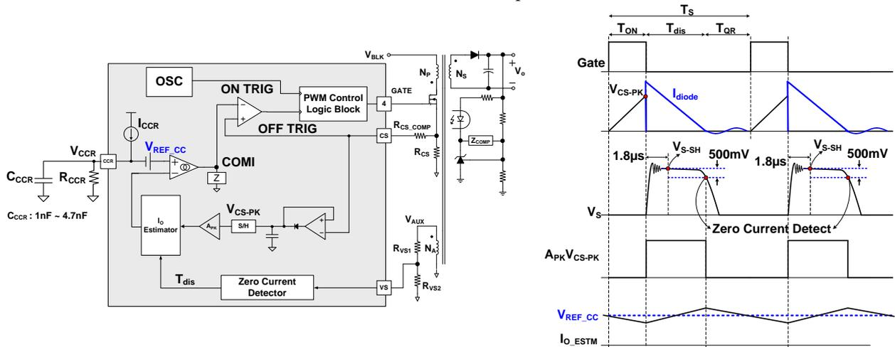
Figure 28 Waveforms for Estimate Output Current
