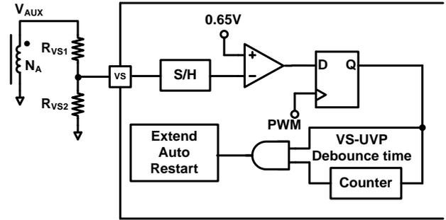
Figure 36 VS-UVP Protection Circuit
