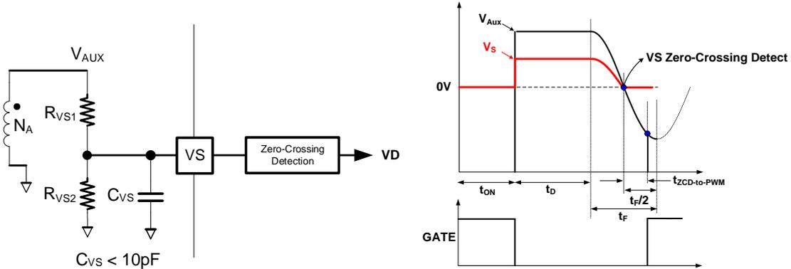
Figure 23 The Valley Detection Circuit and Behavior
