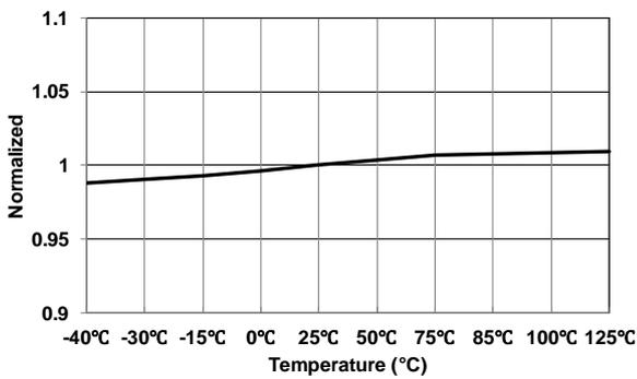
**Figure 7 Maximum Blanking Frequency (f<sub>BNK-MAX</sub>) vs. Temperature**
