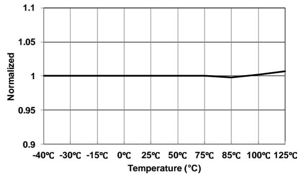
**Figure 6 Brown-In Threshold Voltage (V<sub>Brown-IN</sub>) vs. Temperature**
