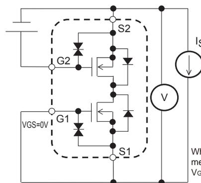
When FET1 is measured, +4.5V is added to V<sub>GS</sub> of FET2.
