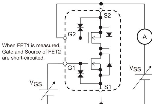
When FET1 is measured, Gate and Source of FET2 are short-circuited.
