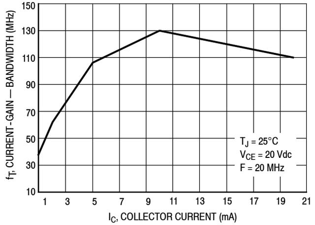
Figure 3. Current-Gain — Bandwidth
