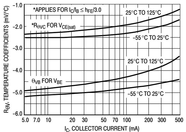
Figure 11. Temperature Coefficients
