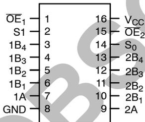
Figure 1. 16-Lead Pinout
