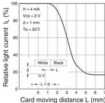
Relative Collector Current vs. Card Moving Distance (2)
