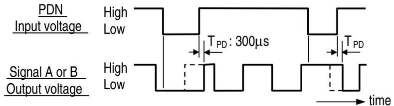
**Note:** Ensure that PDN is Logic High, if the Power Down Function is not used.
