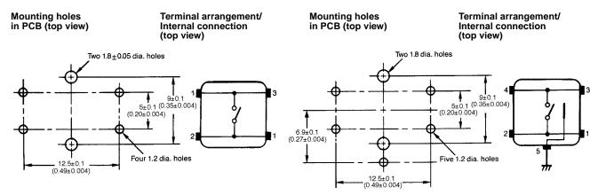
**Note:** Unless otherwise specified, a tolerance of  $\pm$  0.2 mm applies to all dimensions.
