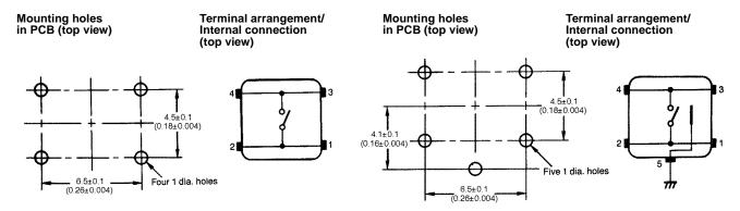
**Note:** Unless otherwise specified, a tolerance of  $\pm\,0.2$  mm applies to all dimensions.
