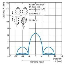
Note: Shading indicates the range in which base bracket will be detected even if switch is open.
