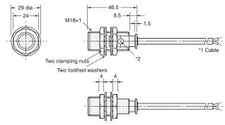
\*1 6-dia. vinyl-insulated round cable with 2 conductors (Conductor cross section: 0.5 mm², Insulator diameter: 1.9 mm), Standard length: 2 m.
