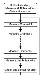
The leadwire compensation measurement and sensor error detection for each input are executed once every N cycles (N = number of active inputs)
