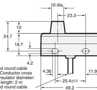
E Models: 4-dia. vinyl-insulated round cable with 3 conductors (Conductor cross section: 0.2 mm<sup>2</sup>, Insulator diameter: 1.2 mm), Standard length: 2 m
