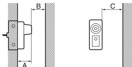
Note: For direct mounting, the distance "C" will equal 0 only in the shaded section of the above left-side section.
