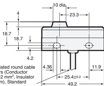
E Models: 4-dia. vinyl-insulated round cable with 3 conductors (Conductor cross section: 0.2 mm<sup>2</sup>, Insulator diameter: 1.2 mm), Standard length: 2 m
